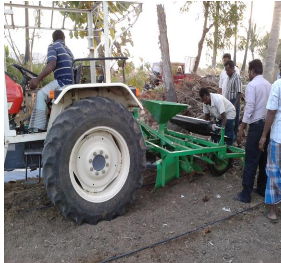
Farmers of a Model Village at Velpadi who have taken up plastic mulching in 20 ha during 2008-09. Tractor with mulch laying machine.
